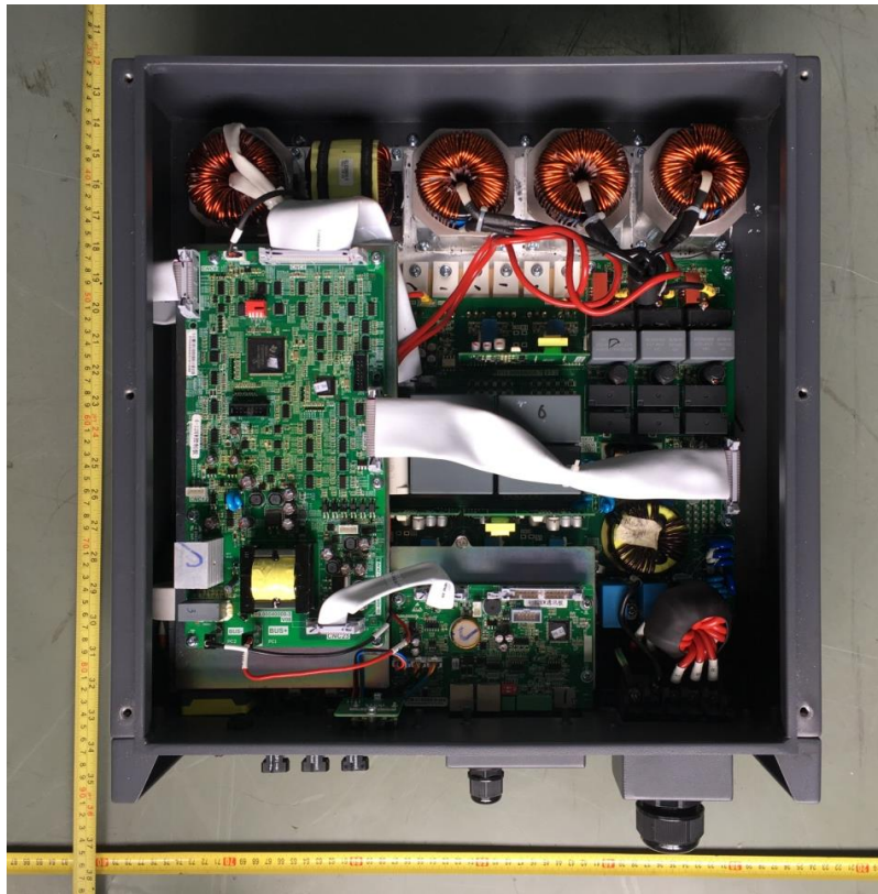
Internal View of Model EVVO 10000TLG23P, EVVO 12000TLG23P
